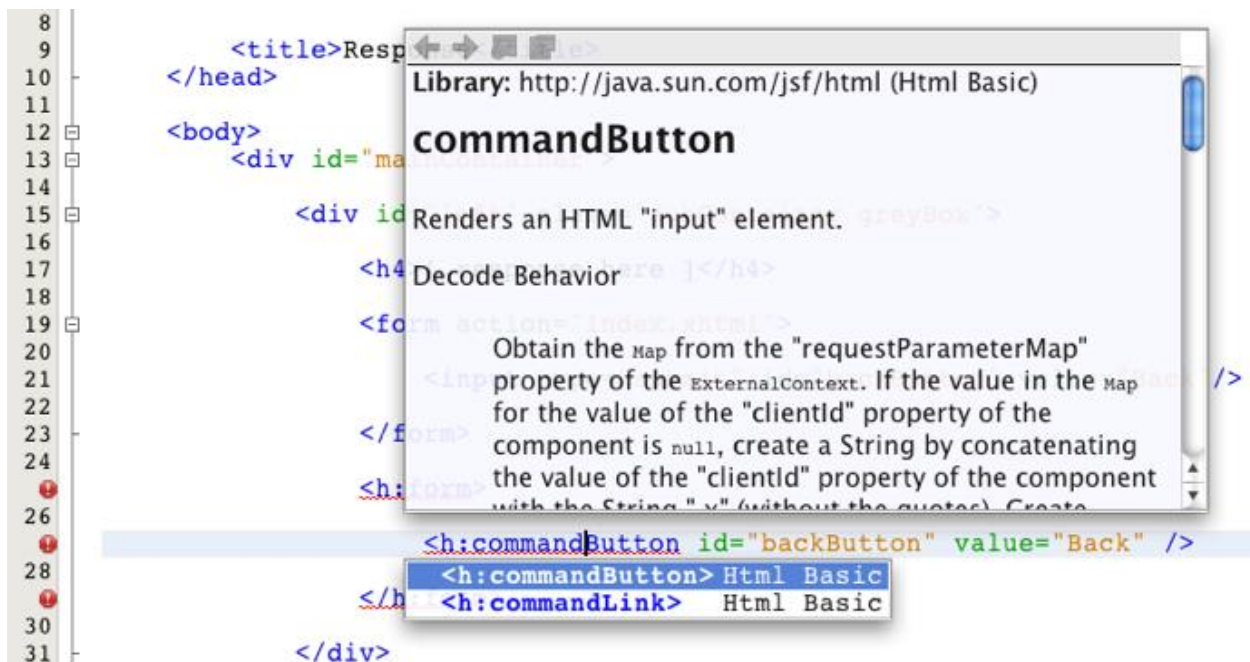
Figure 19. Press Ctrl-Space to invoke code completion suggestions and a documentation pop-up window
